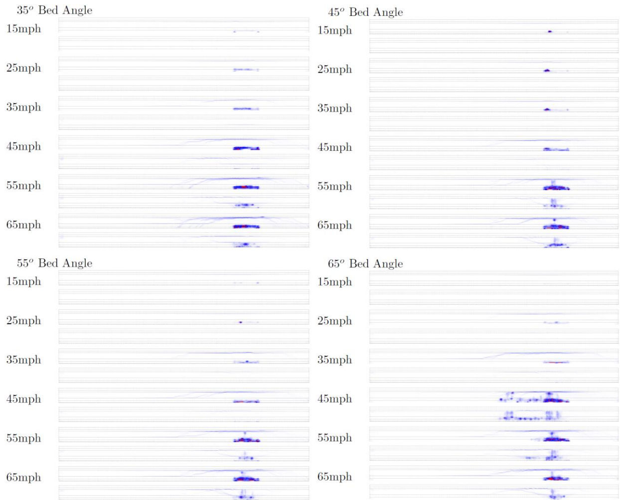
Figure C.9. Maximum principal strain distributions for Scenario 3 impact at quarterpoint (front of exterior girder and rear of exterior girder shown)
