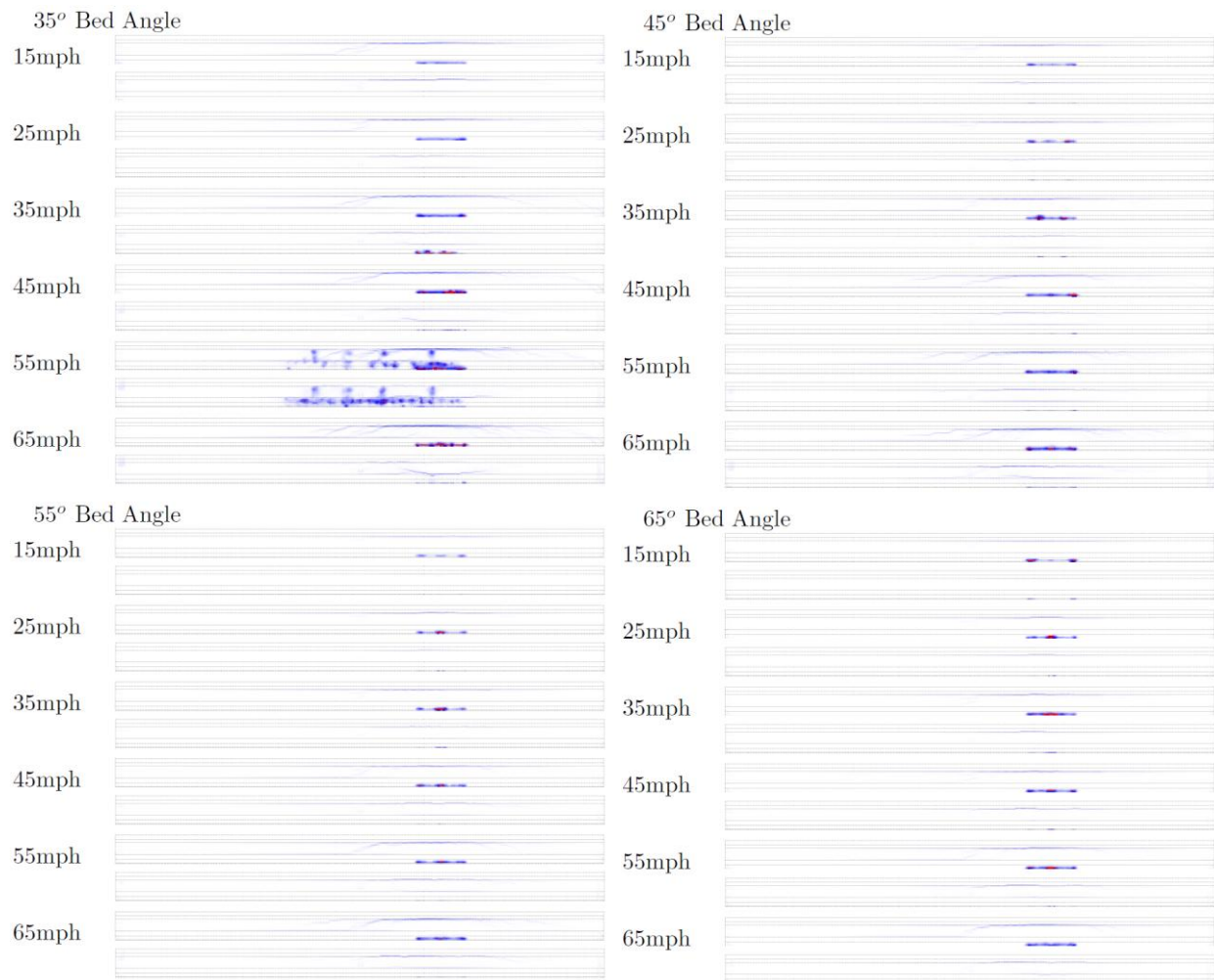
Figure C.11. Maximum principal strain distributions for Scenario 4 impact at third point (front of exterior girder and rear of exterior girder shown)
