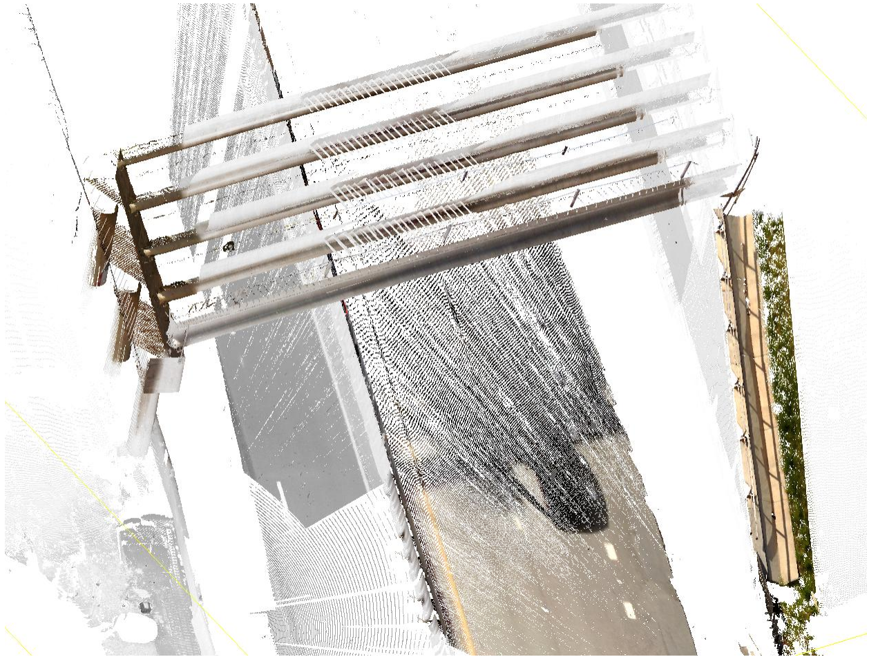
Figure 3.6. Point cloud generated from LiDAR scanning of bridge after incident
