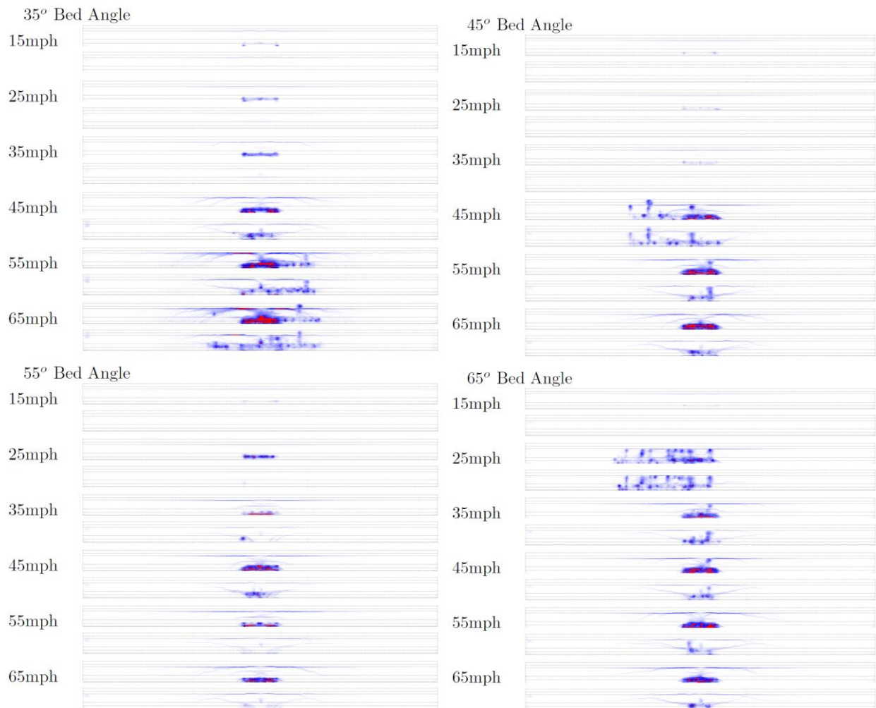
Figure C.7. Maximum principal strain distributions for Scenario 3 impact at midspan (front of exterior girder and rear of exterior girder shown)
