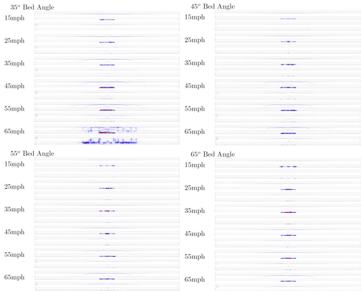
Figure C.10. Maximum principal strain distributions for Scenario 4 impact at midspan (front of exterior girder and rear of exterior girder shown)
