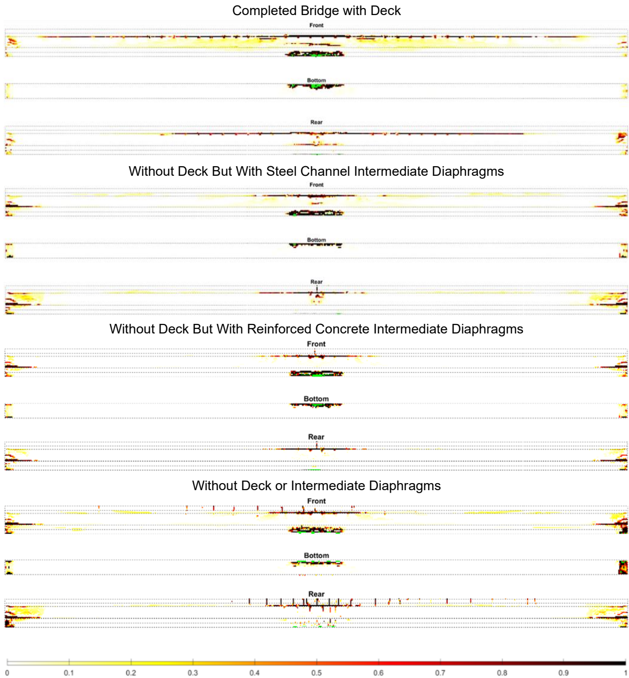
Figure 4.7. Damage predicted for each bridge model following impact from the shield of the dump truck travelling at an initial velocity of 45 mph
