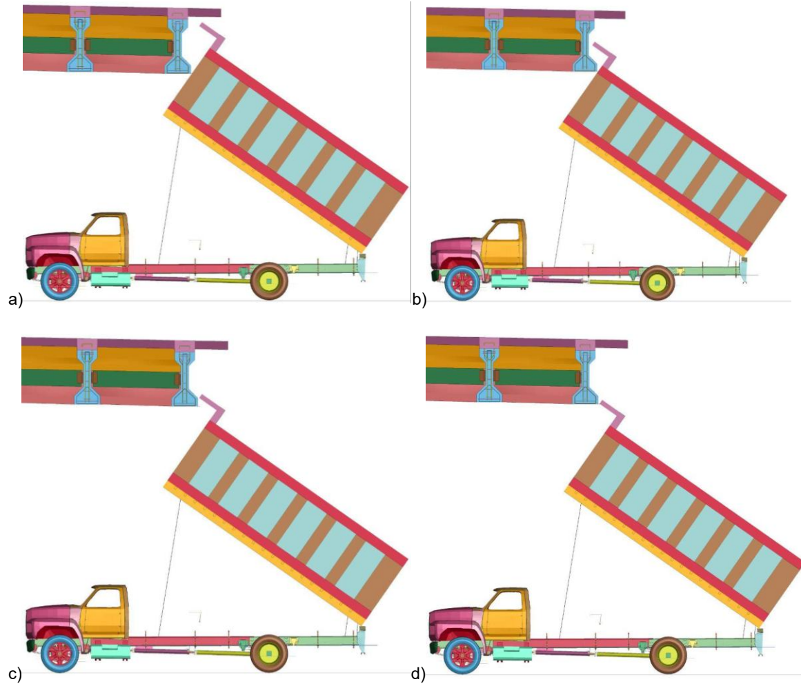
Figure 5.3. Vehicular impact scenarios included in parametric analysis for formulation of simplified damage prediction model: a) Scenario 1; b) Scenario 2; c) Scenario 3; d) Scenario 4
